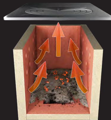
Phase 2: Constant and gradual release of heat even when the fire is already out.
